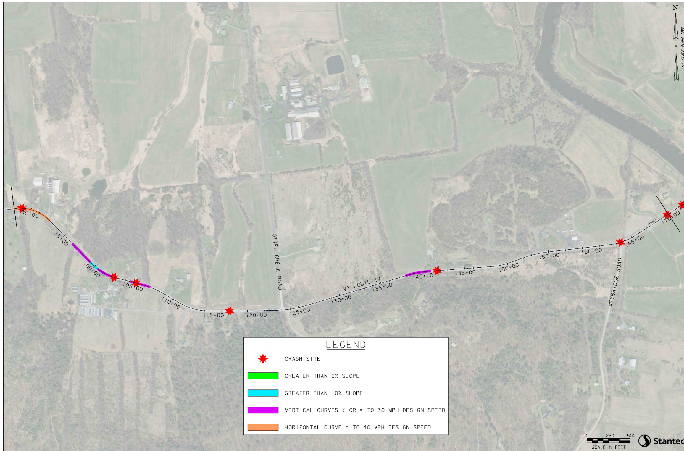
Figure 4-21b VT 17 Design Deficiencies
