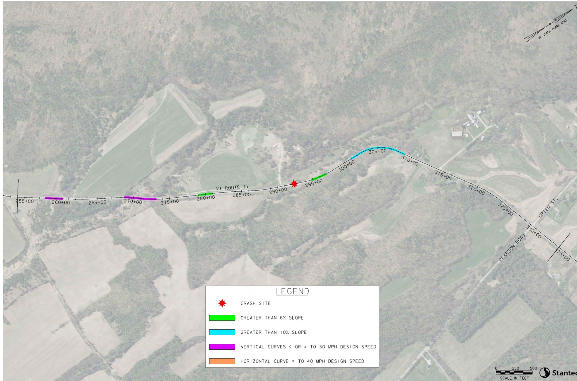
Figure 4-21d VT 17 Design Deficiencies
