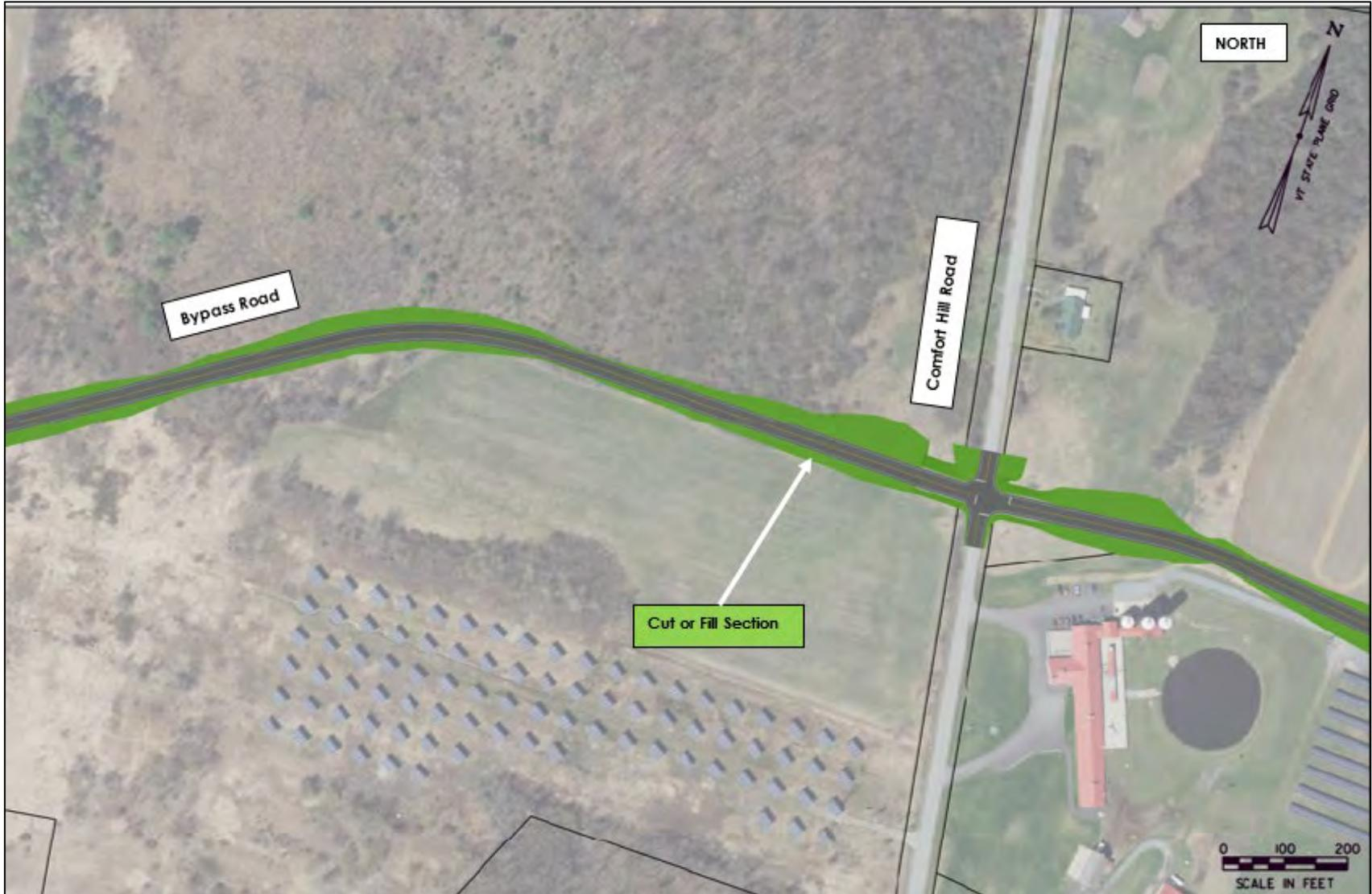
Figure 7-4f Alternative B Concept Plan – Section f
